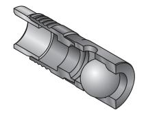
each other. The installation tool can bottom on the insert body. Lee Installation Tools are available for each valve and part numbers are listed on each page. The locking end seals Port A from Port C and retains the valve. During installation, the edge seal at the opposite end is driven into the housing, sealing Port B from Port C.
